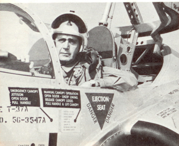
Cockpit view shows open canopy hinge and ejection seat Photo by Ted B. Kiper, Tallahassee, Fla.
